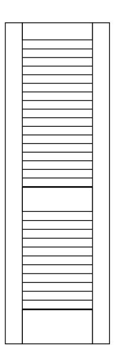
Louver doors and bi-folds are made to order. They feature true stile & rail, doweled construction and square edge sticking. Stiles are built-up to help keep the door stable. Other parts will be solid or glued up as required. Most species are available. We will be happy to customize doors to suit your needs.
